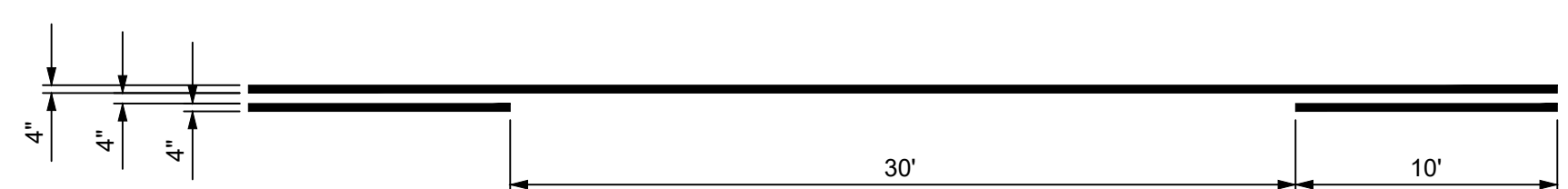
TYPICAL COMBINATION 4" SOLID AND BROKEN LINE DETAIL
