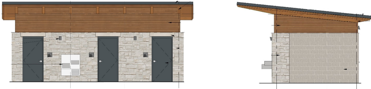
Exhibit 8: Restroom structure front and side elevations.
