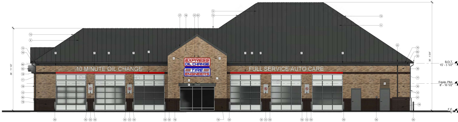
1 01- False Front Elevation (North) 3/16" = 1'-0"
