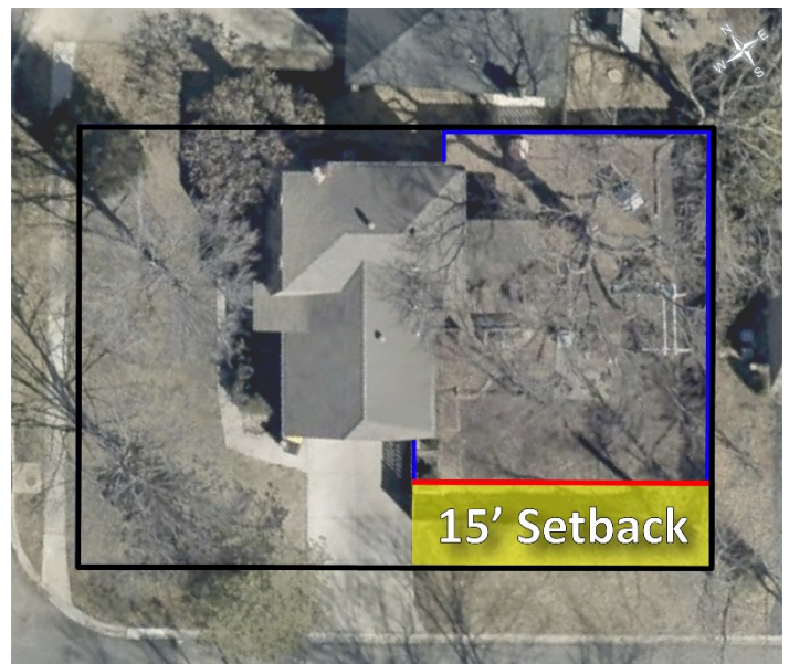
Exhibit 9: Alternative option: 15-foot street-side yard setback per code for open style fences ≤ 4-foot tall.
